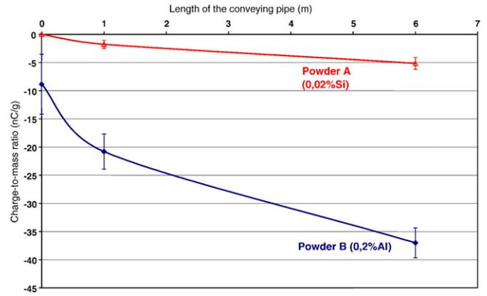
Fig. 7. Influence of the length of the conveying pipe.
