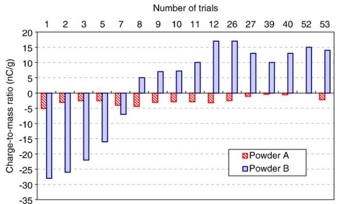
Fig. 8. Influence of the fouling of the pipe on the net charge during the conveying.
