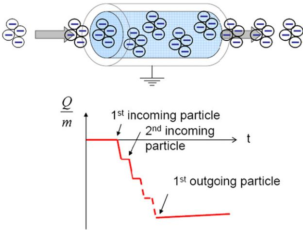
Fig. 5. Powder charge measurement inside a metallic pipe.
