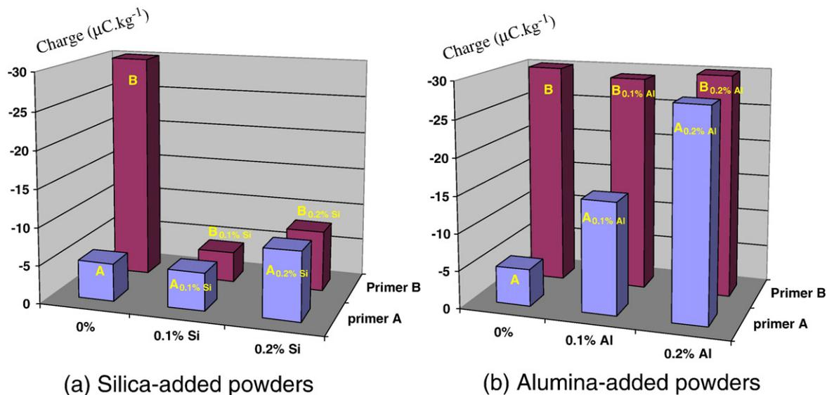
Fig. 9. Net conveying charge measured for laboratory-made powders containing different amounts of flow conditioner (see Table 2).
