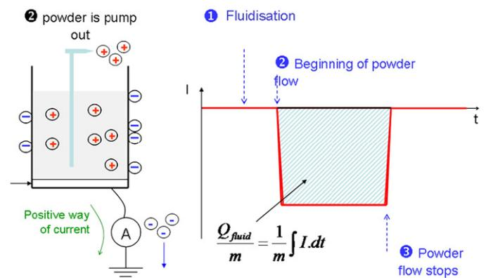
Fig. 4. Fluidisation charge measurement.
